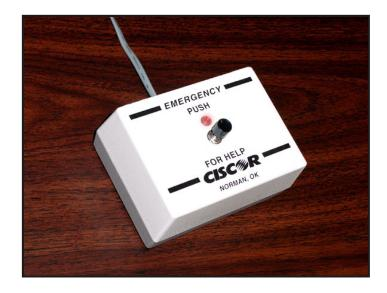
The NS-01 comes with a 10' cord that plugs into a standard RJ-11 wall jack. The cord may be extended with any standard 4 conductor telephone extension cord. The red LED call assurance light, just above the switch, illuminates when the switch is activated. The portability of the NS-01 makes it a good choice for bedrooms and living rooms because it allows for any arrangement of furniture without compromising access to the call switch.
